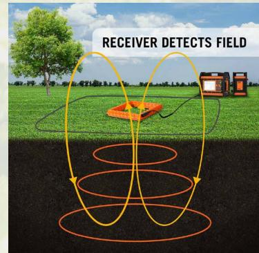
Ground currents create a secondary magnetic field recorded by the Rx loop
