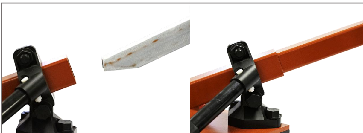
Figure 7: Insert GroundTEM Ralli wings into receivers on the Tx Platform
