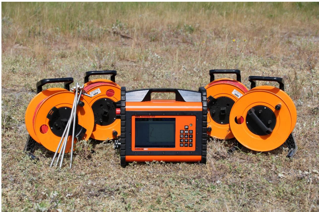
Figure 1 ABEM Terrameter VES and selected accessories
