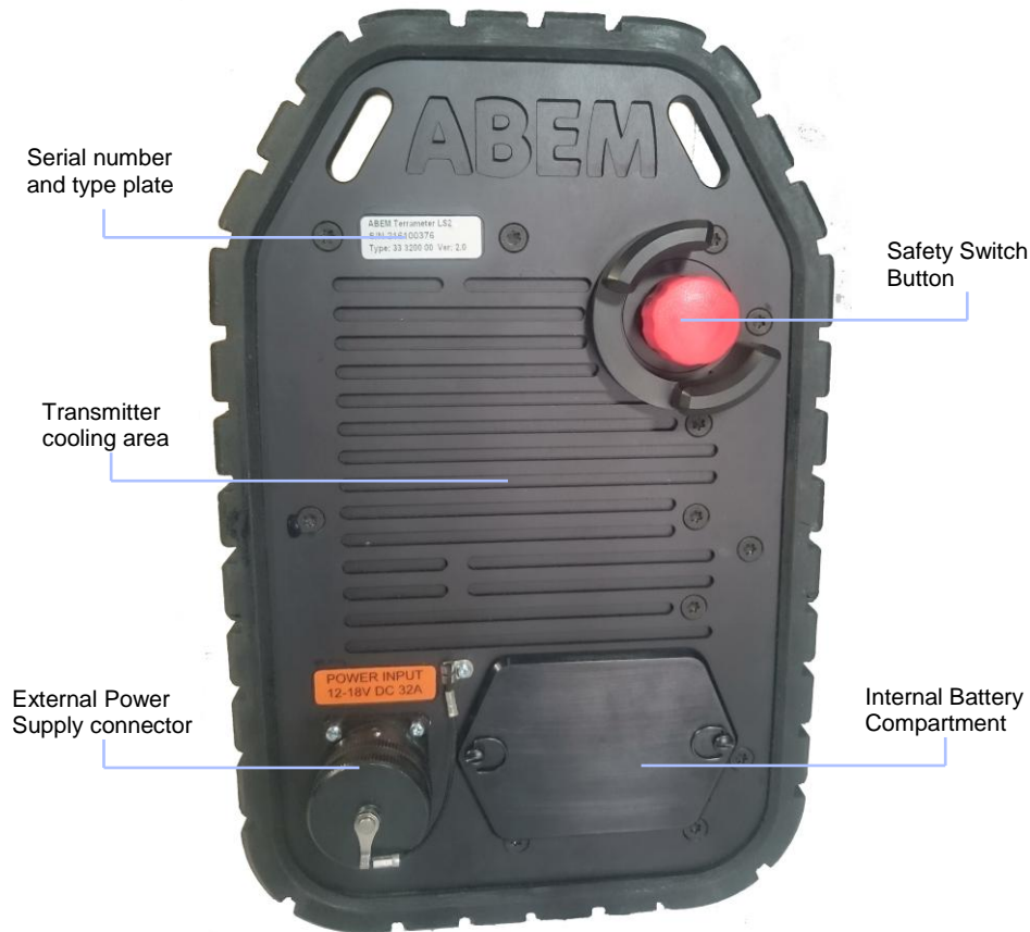
Figure 4 The power panel of a Terrameter VES / VES MAX
