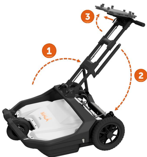
Figure 1. Unfold handle and lower the support arms. Pull MALÅ lanyard to unfold laptop holder.
