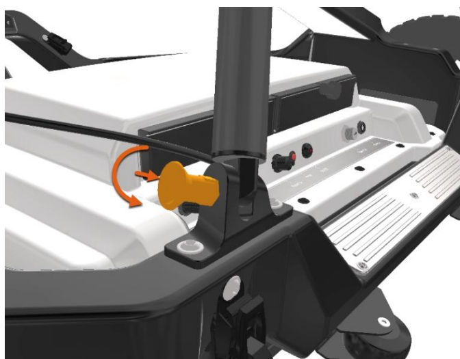
Figure 2. Lock the plunger by rotating the knob and pushing it in to secure the support arms.
