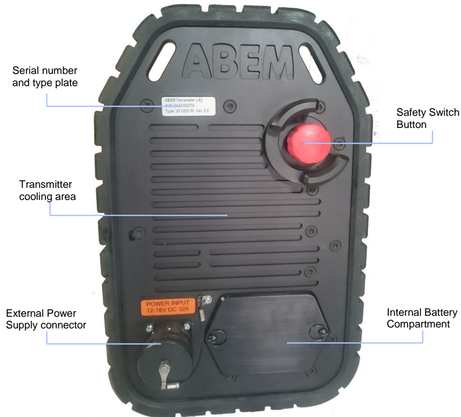
Figure 4 The power panel of Terrameter LS 2
