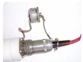
Keep connectors dry and clean. **Poor connector handling and maintenance are the main causes of cable failure.** If using cables with dust caps, always interconnect / cover them to keep them clean and dry during measurements (right).
