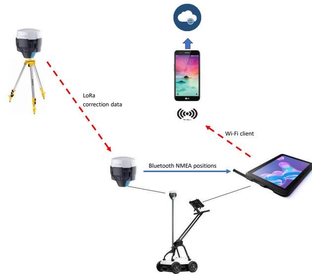
Both Emlid units, the base and the rover, must be equipped with LoRa (Long Range) antennas, to allow correction data to be sent from the base to the rover.
