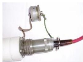
Keep connectors dry and clean. **Poor connector handling and maintenance are the main causes of cable failure.** Always interconnect dust caps to keep them clean and dry during measurements (right).
