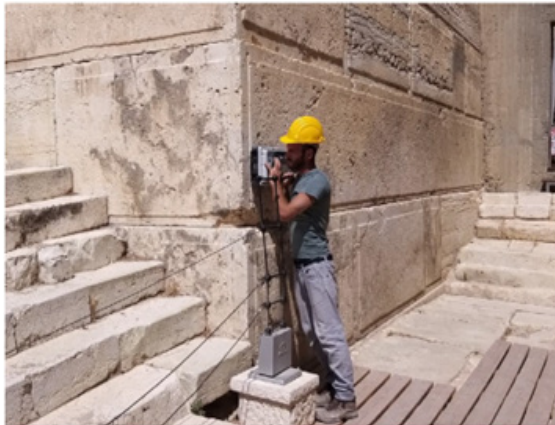
Measurements carried out with the MALÅ GX450 system on different parts of the Western Wall, Jerusalem, Israel, by GeoSense.
