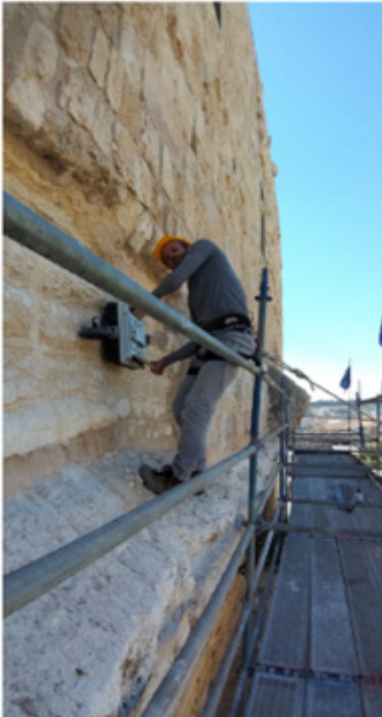
Measurements carried out with the MALÅ GX450 system on different parts of the Western Wall, Jerusalem, Israel, by GeoSense.
