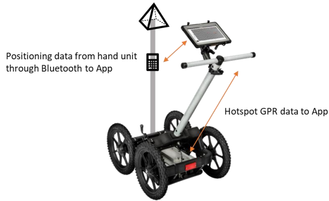
Prism and hand unit on GPR antenna
