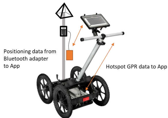
Prism and hand unit with Bluetooth adapter on GPR antenna
