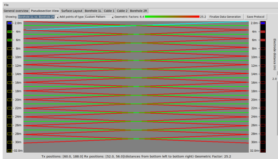
Figure 68 - The pattern is completed by clicking on the bottom electrode of borehole 1L, and the measurements are shown as lines from one borehole to the other
