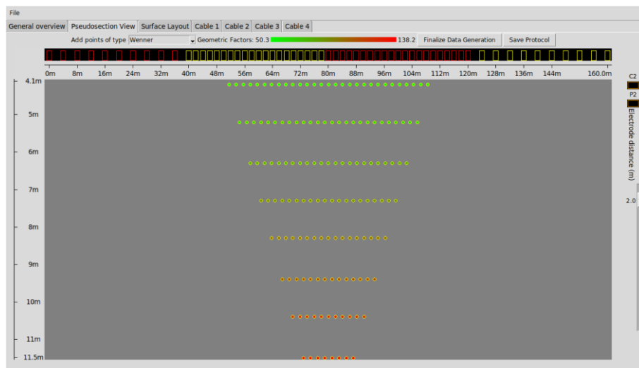
Figure 57 – A Wenner protocol resulting from combined restrictions
