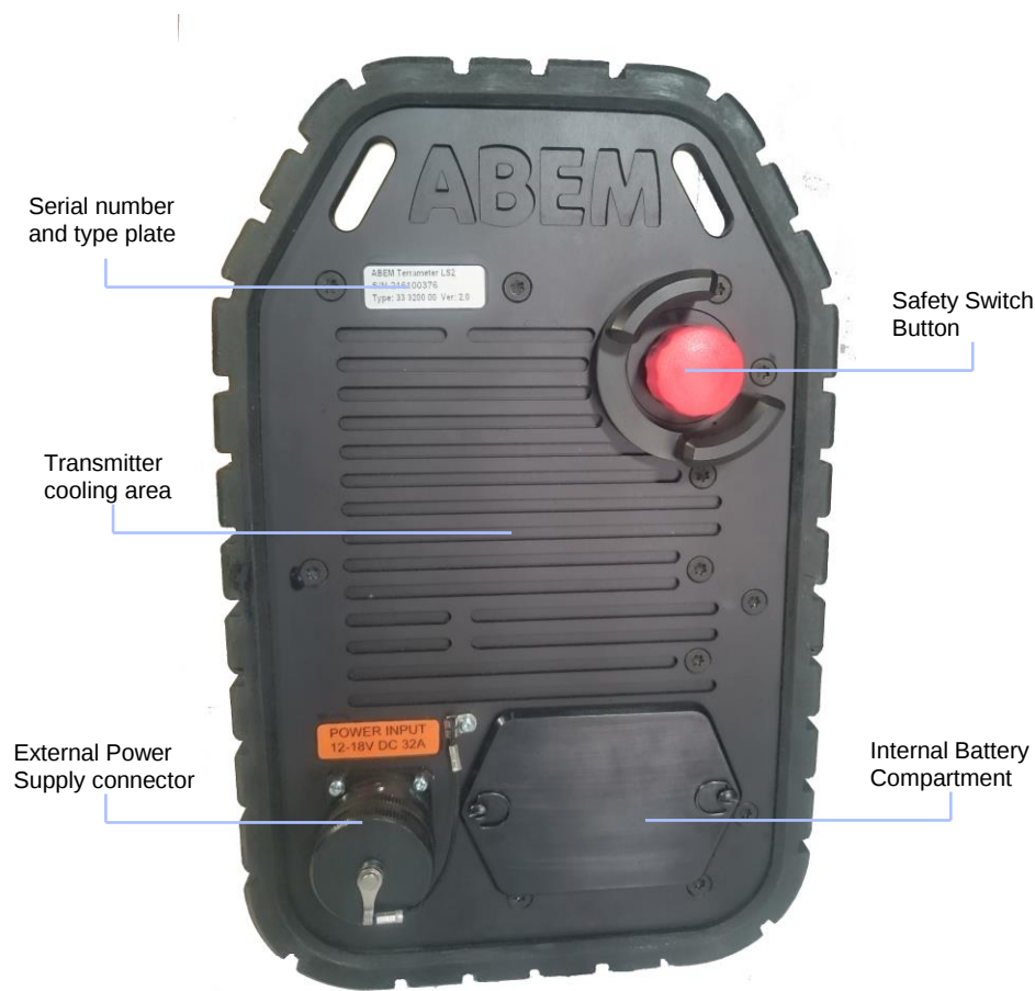
Figure 4 The Power panel of Terrameter LS 2
