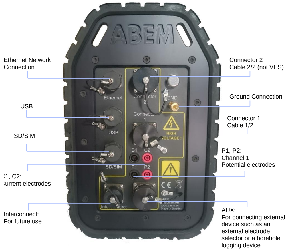
Figure 3 The Connector panel of Terrameter LS 2
