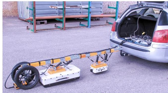
**Note:** The control unit (if using a ProEx) and power supply are placed in the back of the car, and the data acquisition unit (XV Monitor or laptop for ProEx and tablet or GX Controller for GX) in the front seat.
