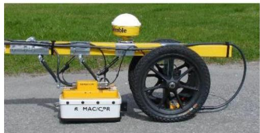
**Note:** The measurement point of the antennas is in the middle of the antenna box, marked with arrows. If two GPR antennas are used simultaneously, it can be best to place the GNSS antenna in-between these two GPR antennas for best positioning of both.
