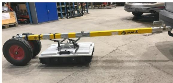
160 MHz GX antenna mounted on the RoadCart.
