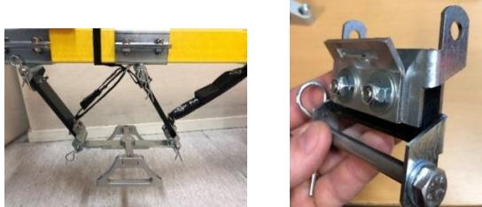
The MALÅ RoadCart is equipped with two different types of holders. The longer type is used for the 450 and 750 MHz antennas and the shorter type for the 160 MHz antenna.
