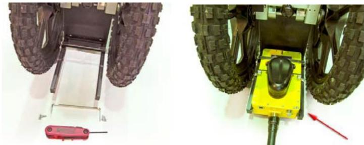
Connect the HF encoder adapter cable between the encoder wheel cable and the HF antenna and connect the HF antenna cable to the control unit used (use extension HF cable if needed).
