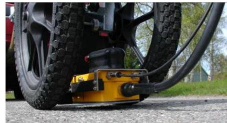
**Note:** Make sure that all cables are tightly attached to the MALÅ RoadCart prior measurements. Use the hook and loop cable ties.
