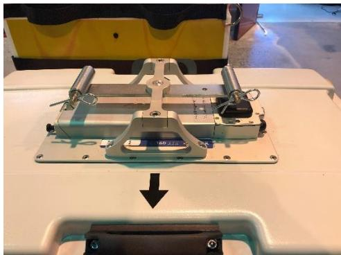
Both holders are attached to the antenna with 4 screws.
