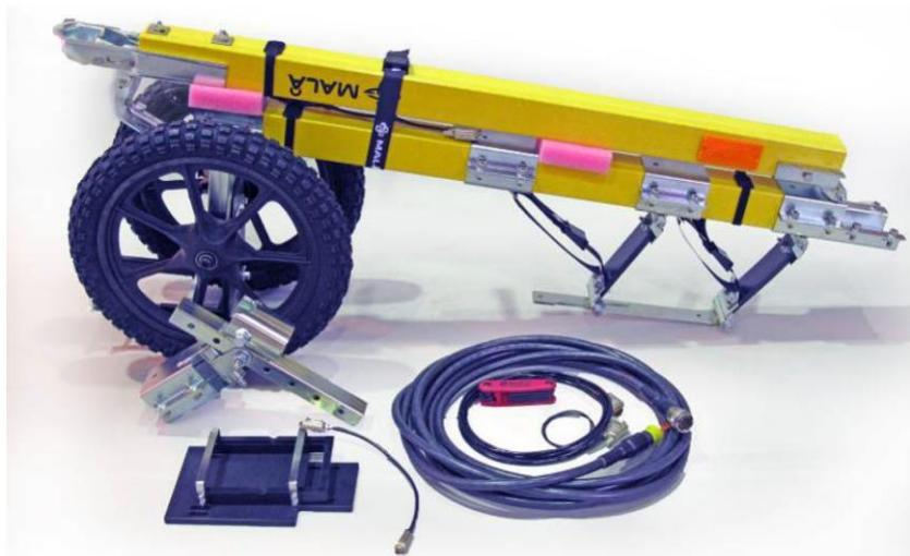
**Note:** Unfold the yellow beam and fasten it with four screws before you mount the antennas.
